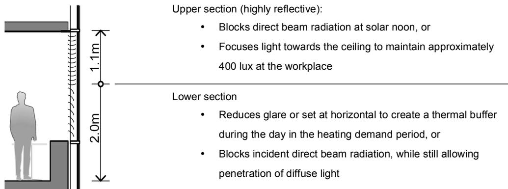
**Figure 4: System B shading applied to the north and east facade**
