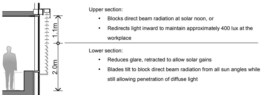
Figure 3: System A shading applied to the north and east facade
